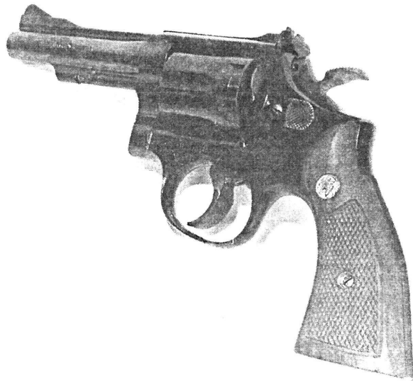
Figure 1-5. Smith and Wesson Combat Masterpiece Caliber .38 Revolver, Model No. 15, Left Rear View
