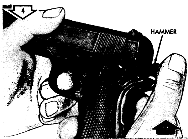
COCK HAMMER FOR REMOVING/INSTALLING SLIDE GROUP.
