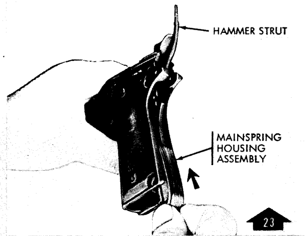
PARTIALLY INSTALL MAINSPRING HOUSING ASSEMBLY TO HOLD SEAR SPRING IN POSITION.
