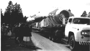
Sc-3: An Atlas E Missile on a specially built trailer being delivered to one of the Fairchild AFB Missile sites. (Source: Courtesy of Richard Mellor).
