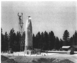
View of Atlas-E ICBM Serial #58-7135 (19E) raised and GOXing ("breathing") at LC 567-9, Reardan/Long Lake, WA., 22 July 1961. (Convair/General Dynamics Photo) Image courtesy of www. Silsoworld.com
