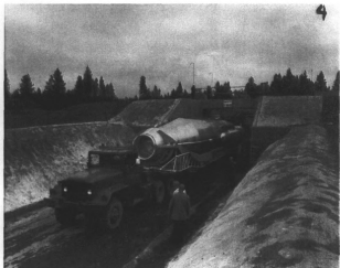
Carefully backing up Atlas E into launcher at Reardan Site. Image courtesy of www. Silsoworld.com
