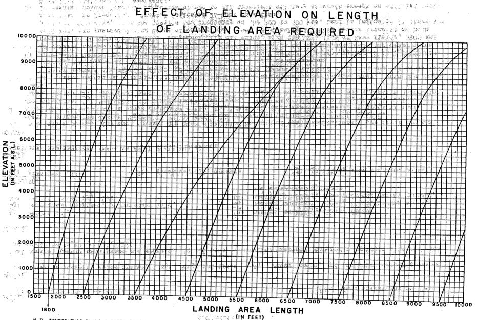
N. B. TEMPERATURE PLAYS A SURPRISINGLY MAJOR PART IN DETERMINING THE EFFECTIVE LENGTH OF A RUNWAY. THE LENGTH OF RUNWAY REQUIRED MAY BE INCREASED, IN EXTREME CASES, BY AS MUCH AS 40% BY TEMPERATURE ALONE. WHILE THE EFFECTIVE RUNWAY LENGTH STEMS MAINLY FROM THE FACTORS OF ELEVATION AND TEMPERATURE, IT IS ALSO INFLUENCED BY THOSE OF GROSS WEIGHT OF PLANE, PILOT TECHNIQUE, AND RUNWAY SURFACE CHARACTER-ISTICS. AS A RULE, THE HIGHER THE TEMPERATURE AND ELEVATION, THE LONGER THE LANDING AND TAKE OFF.
